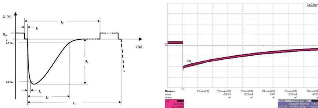
**Figure 6: ISO 7637 Pulse 1 voltage and timing details (spec requirement on the left, actual waveform on the right).**
