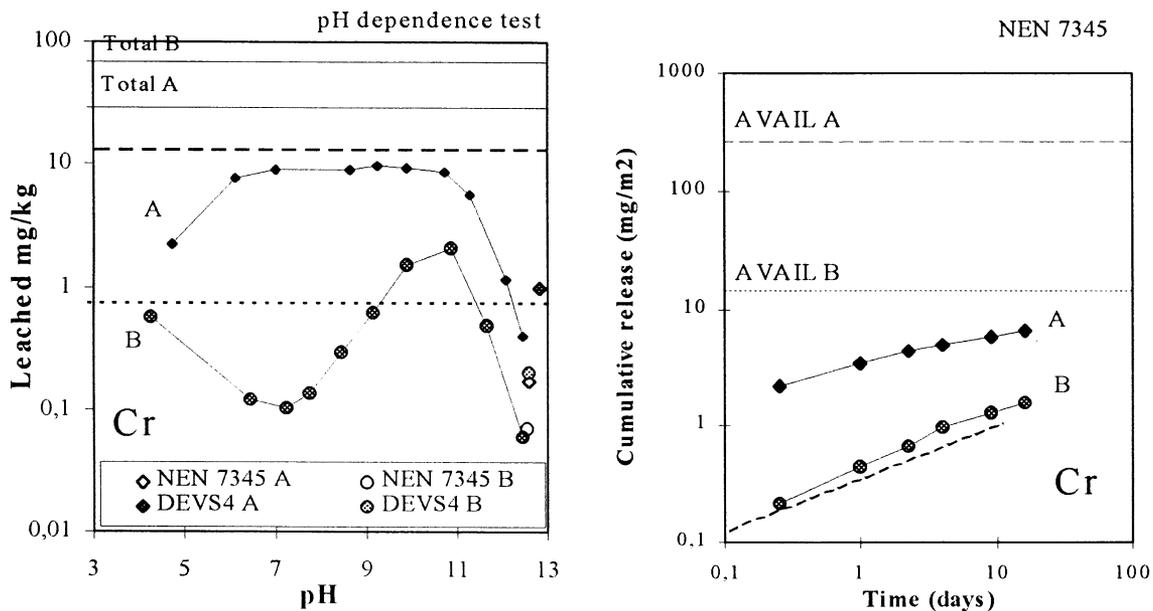
Fig. 7. Comparison and interrelations between leaching tests for Cr from cement mortars.
