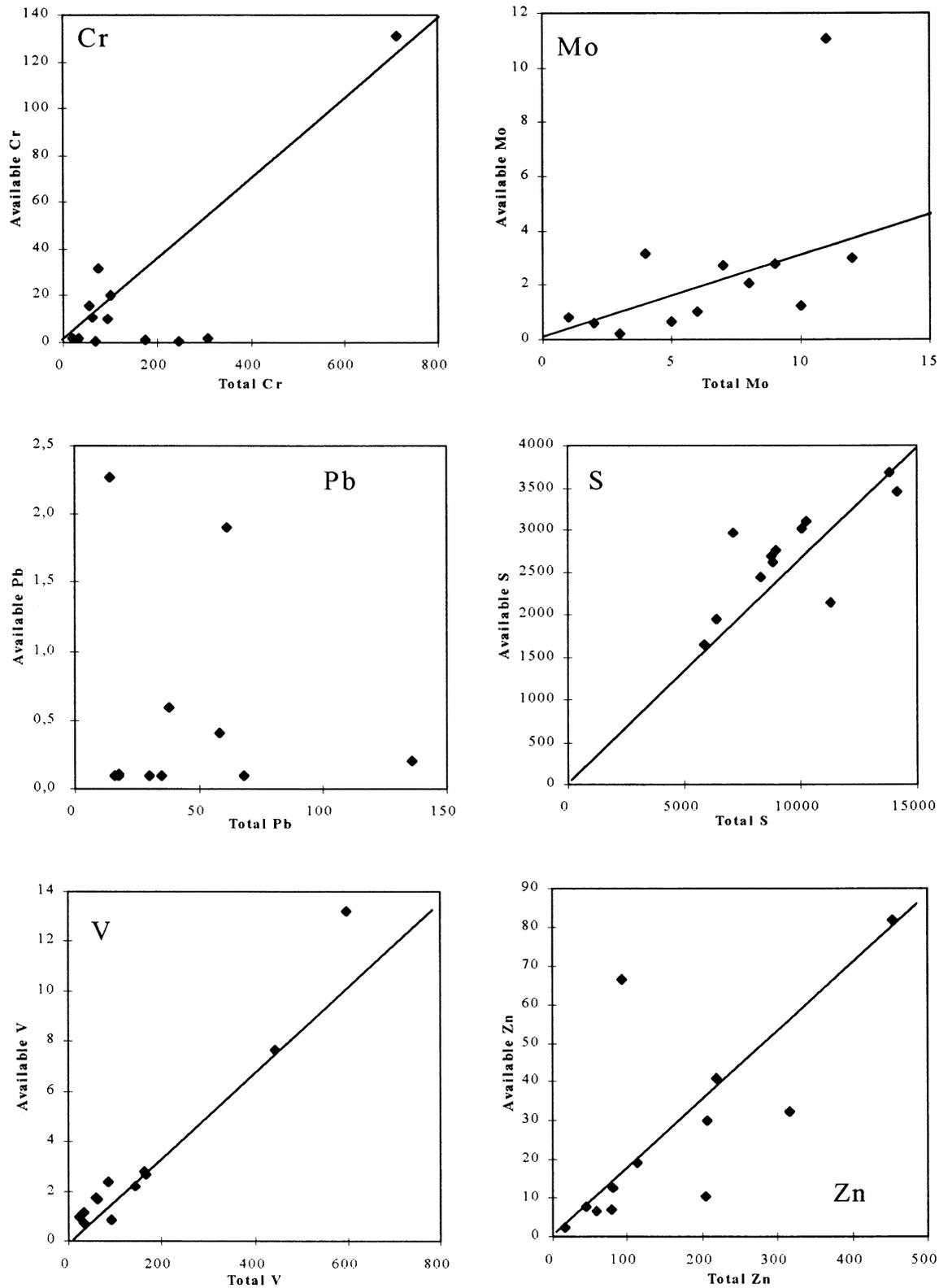
Fig. 3. Correlation between total and availability for Cr, Mo, Pb,S, V, and Zn on all cements (mg/kg).
