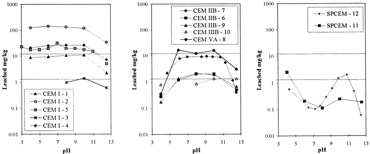
Fig. 9. Consistent leachability of chromium from 12 cement mortars as a function of pH (after crushing to <2 mm; L/S=10; 24 h). BSB categories I and II are regulatory limits according to the Dutch Building Materials Decree.
