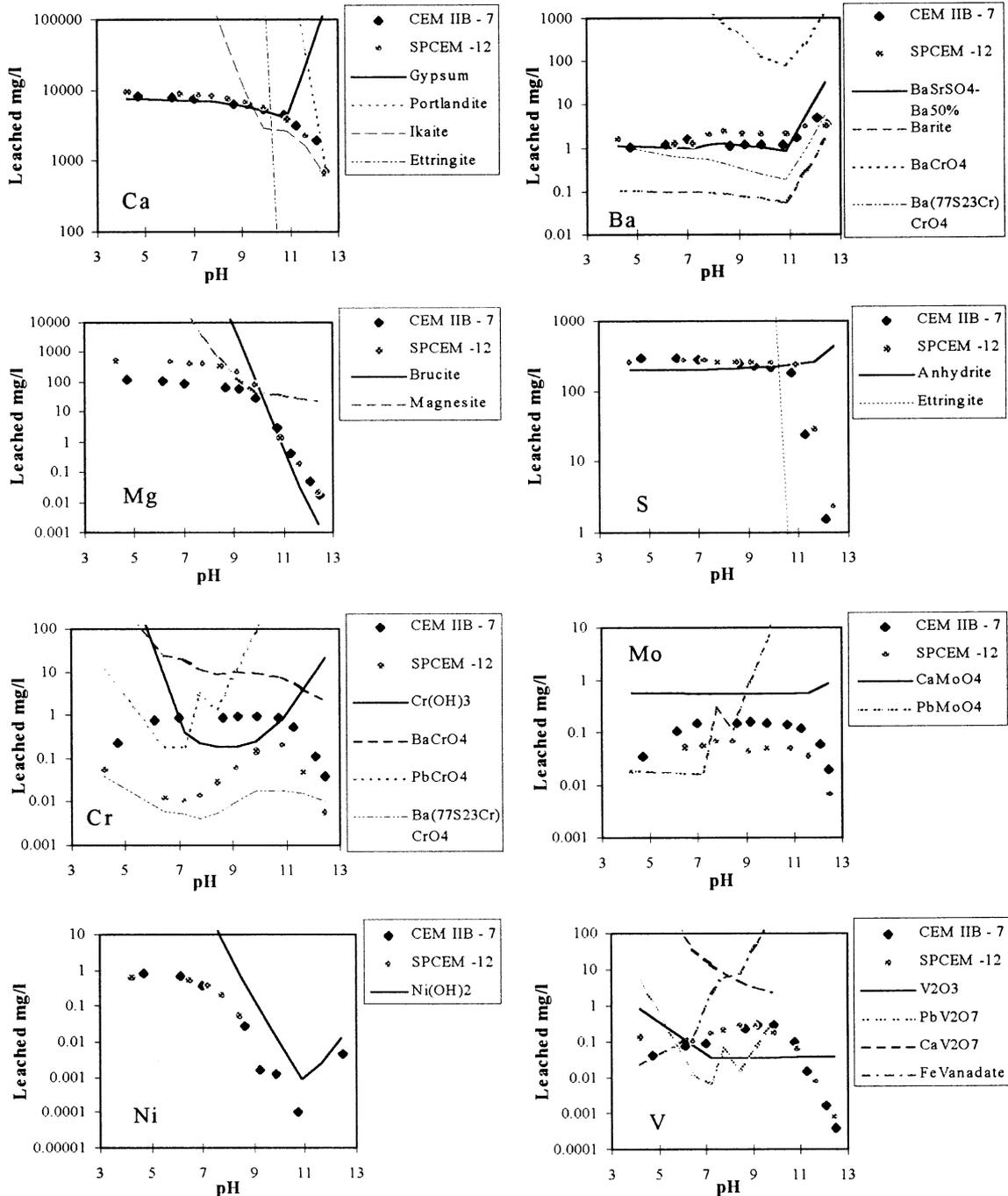
Fig. 10. Geochemical modeling of crushed cement mortars using MINTEQA2.
