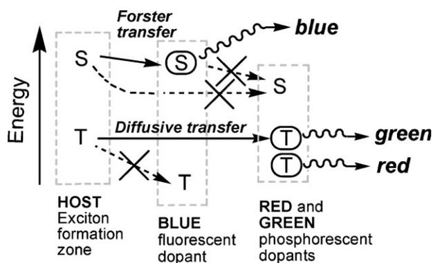
**Figure 2.** Proposed energy transfer mechanisms in a fluorescent/phosphorescent WOLED. This illustrates the separate channels for triplet (T) and singlet (S) formation and transfer directly onto their corresponding emissive dopants. Modified from Reference [37].
