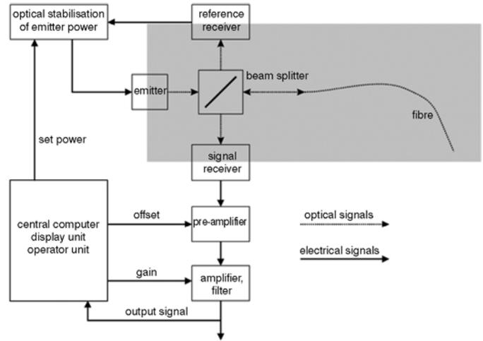
Fig. 2 Schematic diagram of opto-electrical unit and sensing fibre
