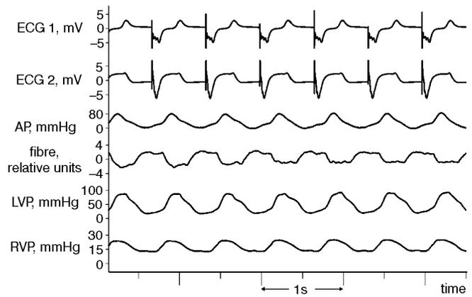
Fig. 7 Fibre signal during contraction and relaxation of pig heart. Epicardial electrocardiogram and intracardial electrocardiogram: ECG 1 and 2; fibre signal: fibre; aortic pressure: AP; left ventricular pressure: LVP; and right ventricular pressure: RVP
