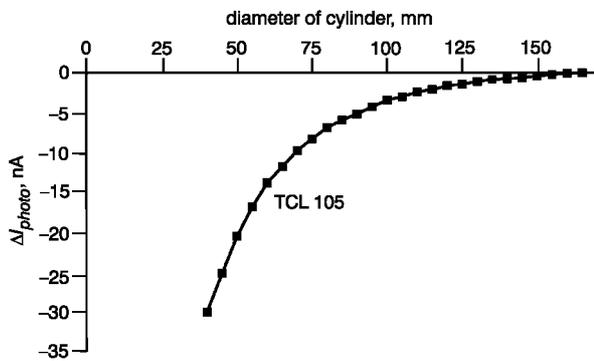
Fig. 5 Change in photo current as function of bending diameter for TCL 105 fibre
