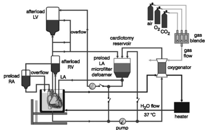
Fig. 6 Isolated working pig heart. RA = right atrium; LA = left atrium; RV = right ventricle; LV = left ventricle
