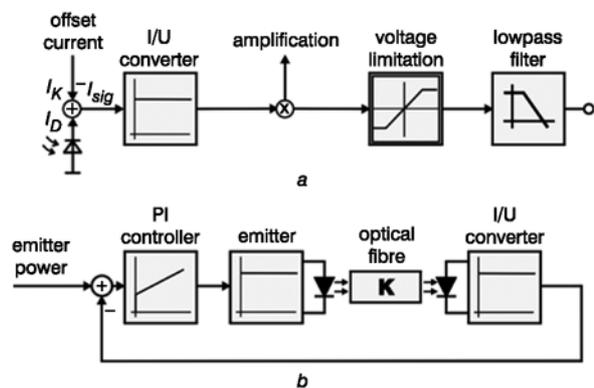
Fig. 3 (a) Diagram of receiver circuit. (b) Power stabilisation circuit of emitter diode
