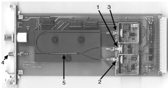
**Fig. 4** Extracorporeal opto-electrical unit. 1: emitter; 2: signal receiver; 3: reference receiver; 4: connector for fibre; 5: coupler/beam splitter
