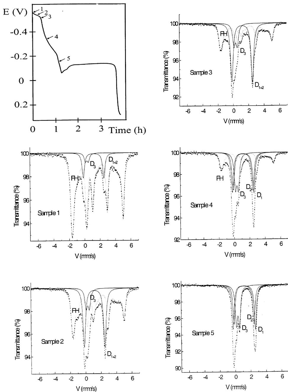
Fig. 1. Mössbauer spectra measured at 20 K of samples 1 to 5, at various stages of the oxidation of ferrous hydroxide into  $\text{GR}(\text{Cl}^-)$  and corresponding  $E$  vs time curve showing the location of the various samplings (the potential axis is downward). TMS:  $\cdots$  experimental curve;  $\text{—}$  elementary quadrupole doublets;  $\text{---}$  global computed curve.
