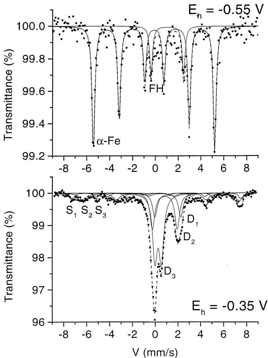
Fig. 4. Mössbauer spectra measured at room temperature of the electrochemically induced corrosion products of  $\alpha$ -iron in a 1 M KCl solution of pH about 9, compared to that of standard  $GR(Cl^-)$ .  $\cdots$  experimental curve;  $—$  elementary quadrupole doublets;  $---$  global computed curve.
