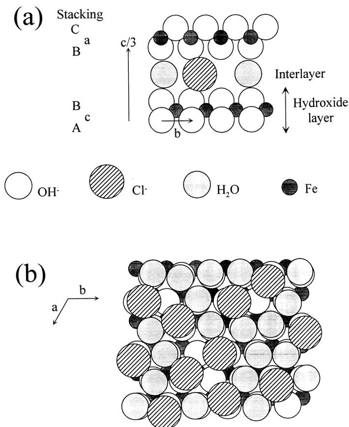
Fig. 6. Crystal structure of  $\text{GR}(\text{Cl}^-)$ . (a) Stacking sequence. (b) Disposition of water molecules and chloride ions in an interlayer viewed along  $[001]$ . Only one interlayer, one  $\text{OH}^-$  and one Fe layer below it are represented.
