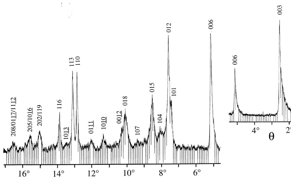
Fig. 5. X-ray powder diffraction pattern of GR(Cl<sup>-</sup>). (MoK $\alpha_1$  radiation,  $\lambda = 0.070930$  nm).
