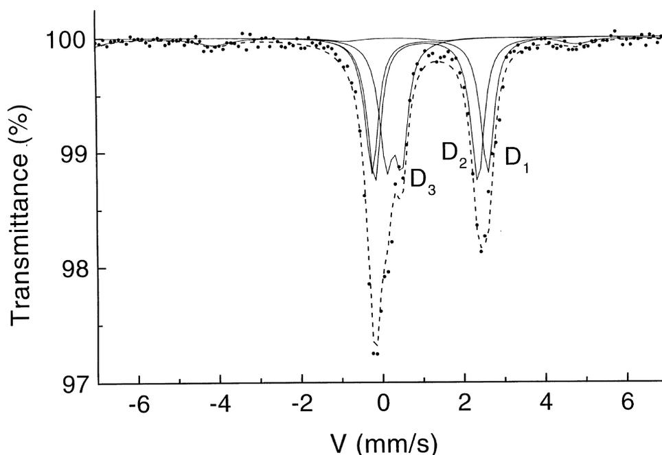
Fig. 2. Mössbauer spectrum measured at 20 K of GR(Cl<sup>-</sup>) precipitated from ferrous and ferric chloride solutions. ··· experimental curve; — elementary quadrupole doublets; — global computed curve.
