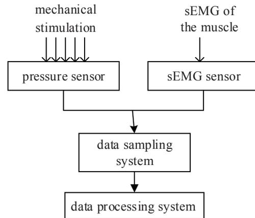
Fig 1. Detection principle of multi-information sampling system
