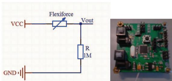
Fig 2. The circuit schematic (left) and circuit board (right) of the detection circuit.
