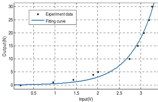
Fig 3. The calibration curve of Flexiforce
